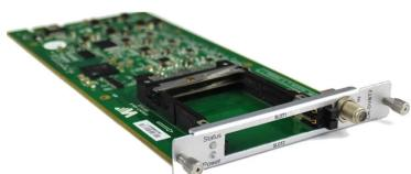
**GX-4T2CI-BP-00** receiver module is equipped with one RF coaxial input connector (F Female) and two PCMCIA Common Interface slots. The module is able to tune **up to four DVB-T/T2 digital terrestrial multiplexes**, decrypt the scrambled programs through the C.I. slots and share and pool the contents to the **GALAXIA** main chassis.
