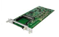
**GX-4C2CI-BP-00** receiver module is equipped with one RF coaxial input connector (F Female) and two PCMCIA Common Interface slots. The module is able to tune up to **four DVB-C digital QAM multiplexes**, decrypt the scrambled programs through the C.I. slots and share and pool the contents to the **GALAXIA** main chassis.
