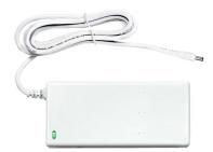
**12V 4A** power supply with **male jack connector** (2.1 x 5.5 x 12mm; inner positive, outer negative) and European plug.
