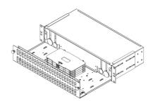
19" 2U rack metal optical drawer for interconnecting up to 48 optical sleeves
