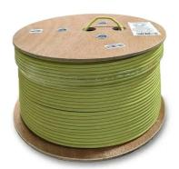
Indoor CAT 6A U/UTP Cca network cable with LSZH sheathing, 305 m skein unwind cable consisting of 4 balanced pairs with AWG 23 flexible red copper conductors. Features meet the requirements of CAT 6A up to 250 MHz according to ANSI/TIA 568.2-D and ISO/IEC 11801 standards. Suitable for 10 Gigabit Ethernet (IEEE 802.3an) applications. Supported PoE applications:
