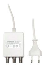
High-efficiency, low-consumption 24V stabilized switchingtype power supply with 1 input, 2 outputs and 100mA delivered current. C-type plug for mains connection.
