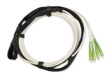
Pre-terminated optical cable in single-mode 9/125 fiber for indoor use, bend insensitive, with 4 SC/APC connectorized fibers and a PULL traction system, 40 m long.
