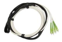
Pre-terminated optical cable in single-mode 9/125 fiber for indoor use, bend insensitive, **with 4 SC/APC connectorized fibers** and a **PULL** traction system, 50 m long.
