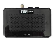
Passive Optical Network Terminal for digital TV signal distribution using the PON network.
