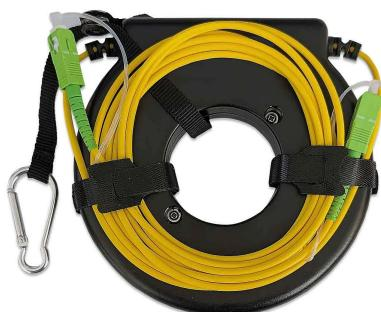
150 OS2 single-mode launch fiber, designed for precision fiber optic testing.
