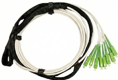
Pre-terminated optical cable in single-mode 9/125 fiber for indoor use, bend insensitive, with **4 SC/APC connectorized fibers** and a **PULL** traction system, 30 m long.
