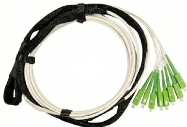
Pre-terminated optical cable in single-mode 9/125 fiber for indoor use, bend insensitive, with 8 SC/APC connectorized fibers and a PULL traction system, 80 m long.
