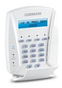
Backlit alphanumeric keypad with liquid crystal display. It enables advanced management of all wired control panels in the Defender system. It is equipped with 4 function keys, with LEDs, freely programmable to enable quick activation of preferred functions.
