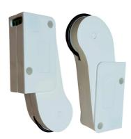
Roller shutter contact, due to its special construction is able to follow the movement of the shutter, because of the built-in tilting rod. The contact is complete with a 4-pole NC terminal block for alarm output and tamper output. The contact is available in two models: white or brown.
