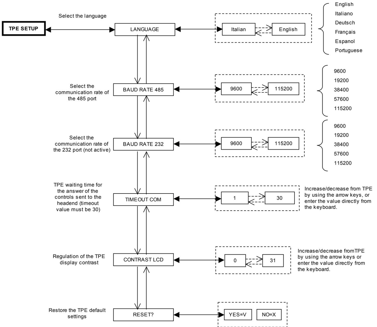
Confirm the settings by pressing the ✓ key; save the settings by pressing the S key after the modules programming.
