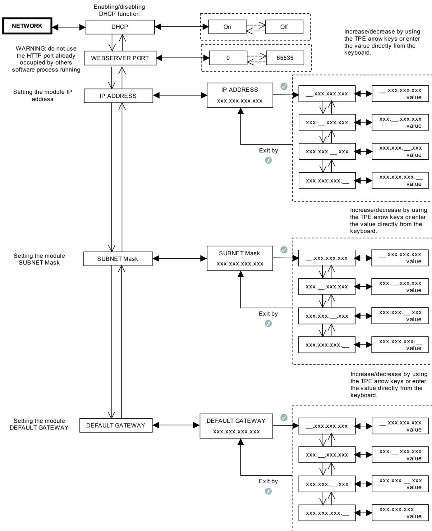
Confirm the settings by pressing the ✓ key; save the settings by pressing the S key after the modules programming.
