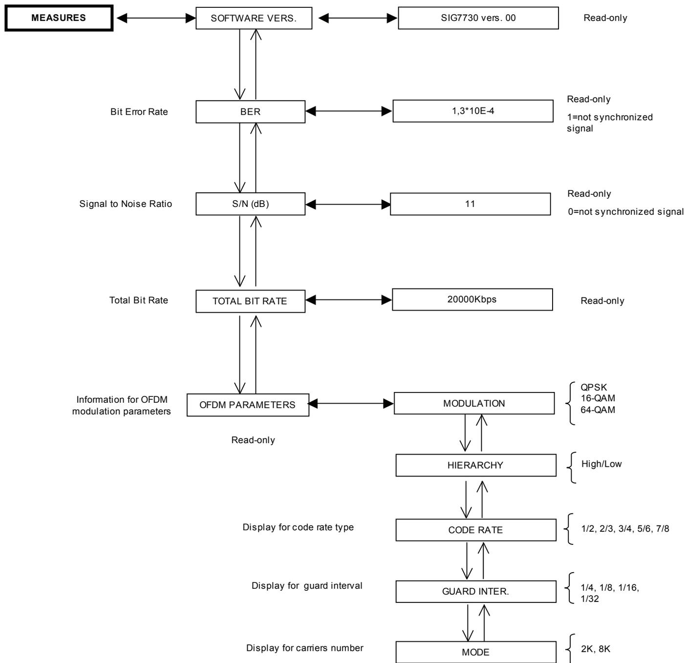
Confirm the settings by pressing the ✓ key; save the settings by pressing the S key after the modules programming.
