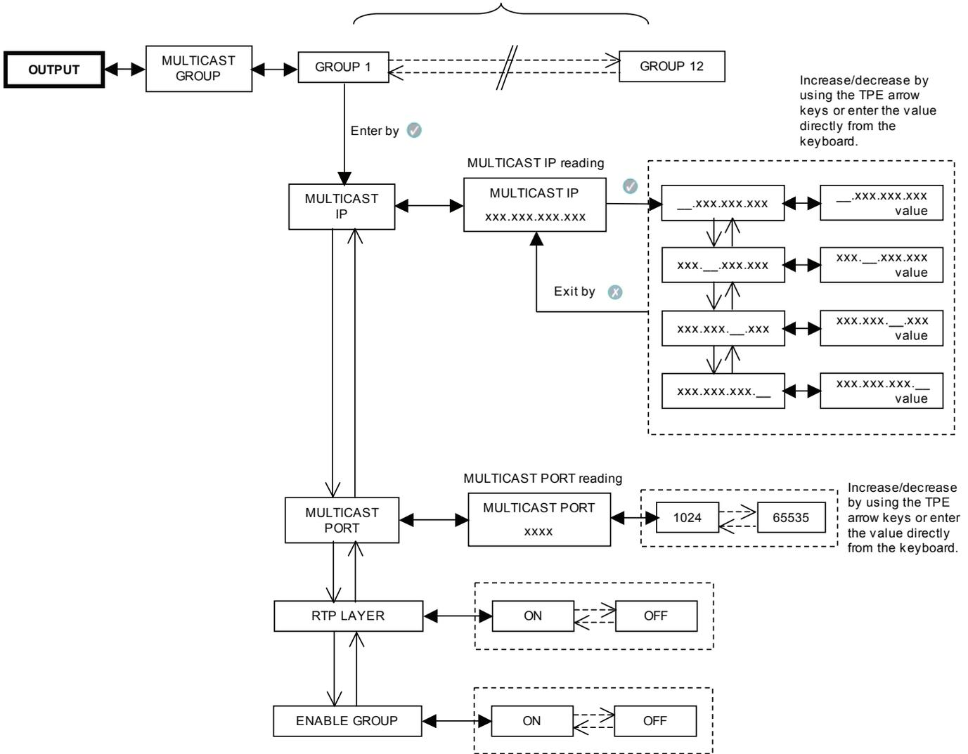
Confirm the settings by pressing the ✓ key; save the settings by pressing the S key after the modules programming.
