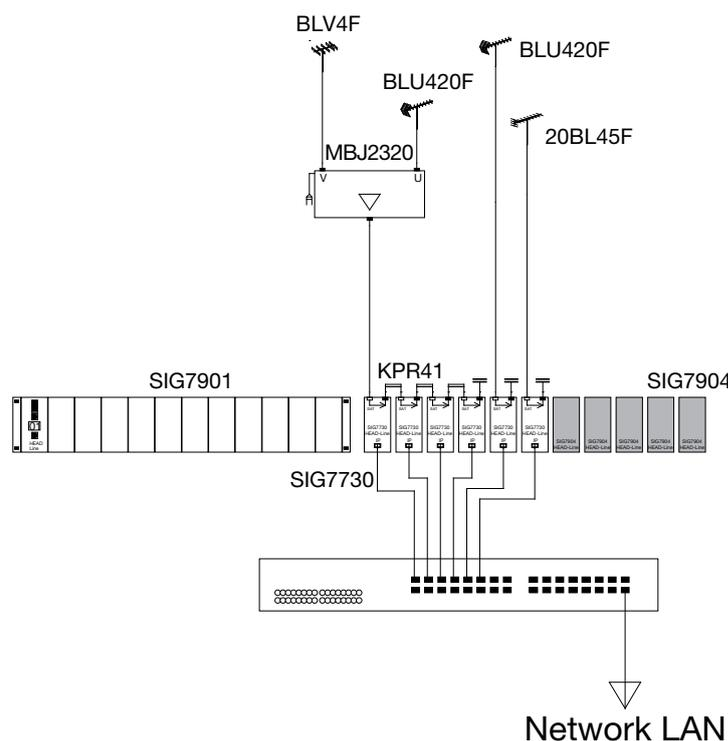
**IMPORTANT:** the installation must be prepared and scaled to support a flow rate equal to at least 100Mbit/s; moreover, so as not to jam the available traffic, all the active devices that will make up the network will have to be able to support **MULTICASTING** features. This verification will be carried out by the administrator of the network where the encoder will be installed.
