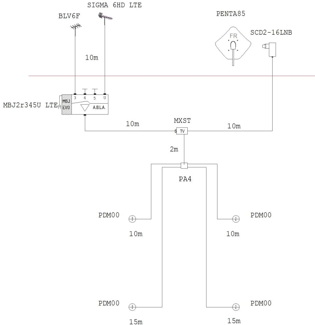
Indication of antennas, antenna holders and preamplifiers from the pole in the scheme is purely indicative, as the choice depends exclusively from the type of TV signal received in the zone of construction of the plant and the structure of the building. The present scheme of proposed maximum does not constitute a project to be drafted by designer enabled, stable. The present scheme of maximum proposed does not constitute a project that must be drawn up by a qualified designer.
